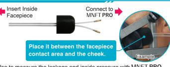
Use to measure the leakage and inside pressure with MNFT PRO.
